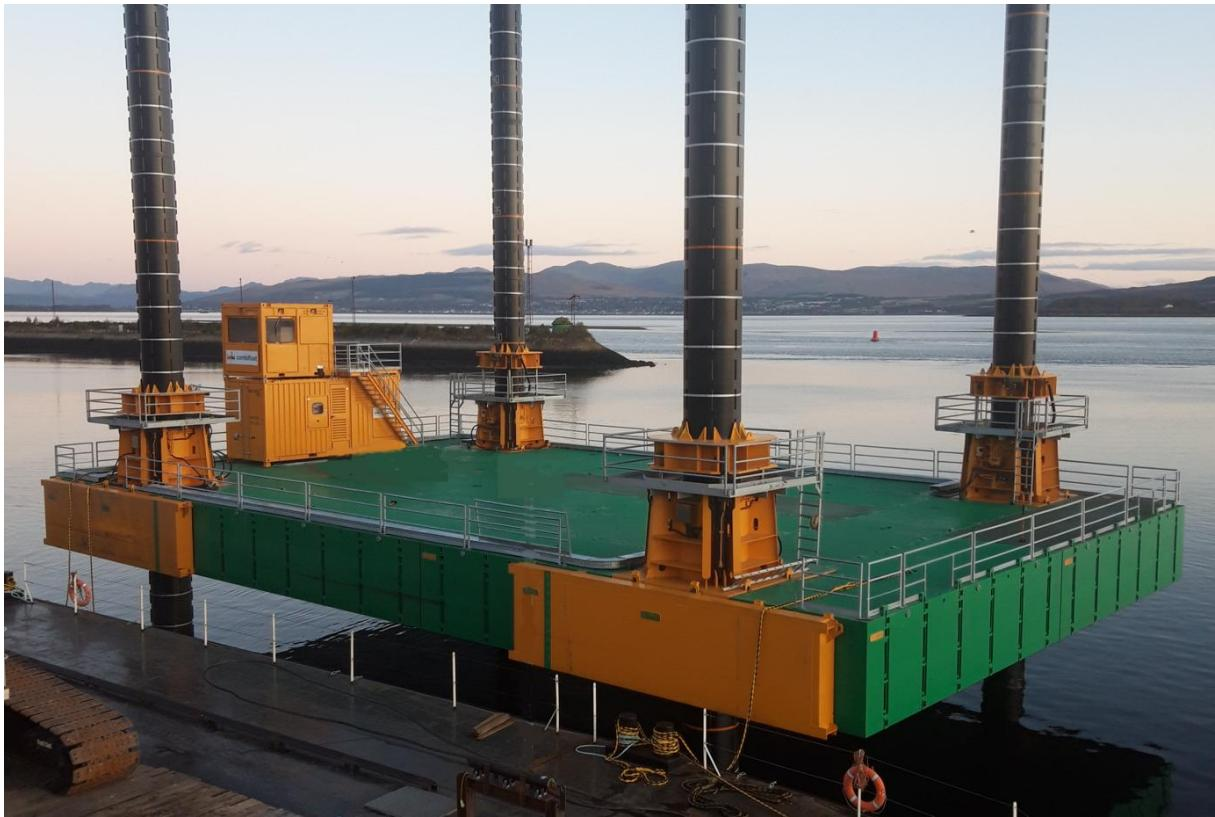
With a variable deck load capacity of 400 mt and an unparalleled 20 mt/m<sup>2</sup> deck strengths, the C-7 is without obstructions on deck. The deck layout can be fully tailored to client's mission equipment and operating method. Depending on soil penetration and waves, the platform can operate in water depths of up to approximately 26 meter, possible more in a moderate environment.
