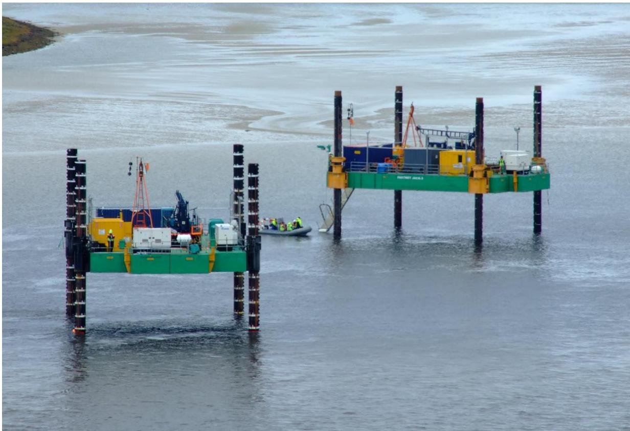
With a 100 mt variable deck load capacity and 15 mt/m<sup>2</sup> deck strength, the C-5 is the platform of choice for geotechnical companies. Over 250 m<sup>2</sup> deck space is usable without obstructions. The deck layout can be fully tailored to client's mission equipment and operating method. To facilitate drilling operations, moonpools or drill slots can be created. This can easily be done by shifting pontoons during assembly or by integrating a drilling slot in a pontoon.
