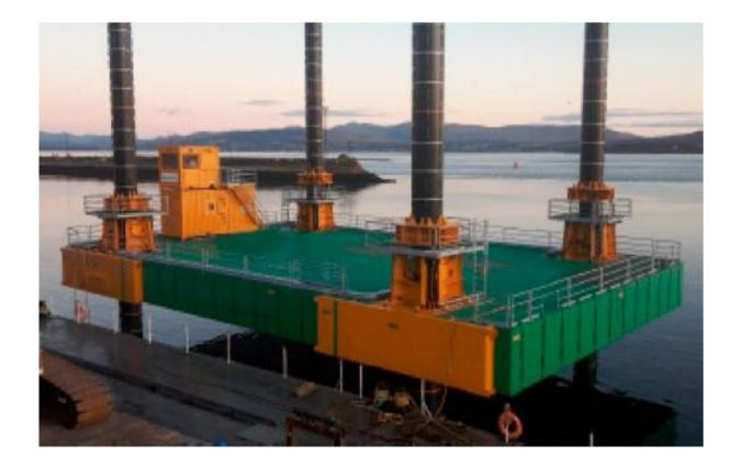
With a variable deck load capacity of 400 tons and an unparalled 15 ton/m² deck strengths, the C7 is without obstructions on deck. The deck layout can be fully tailored to client's mission equipment and operating method. Depending on soil penetration and waves, the platform can cover water depths up to 30 meter, possible more in a moderate environment.
