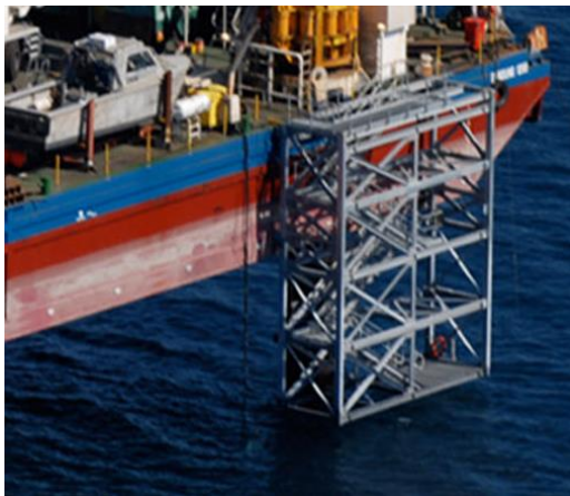
Staircase system (above) installed to hull of jack-up barge – CTV can push on to this system.
