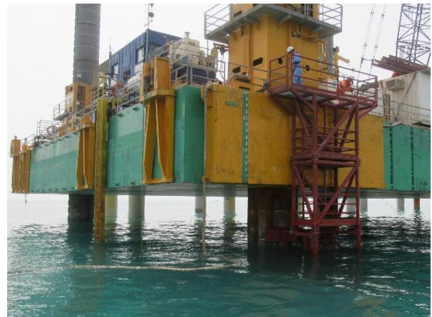
Staircase system (above) installed to hull of jack-up barge – CTV can push on to this system.
