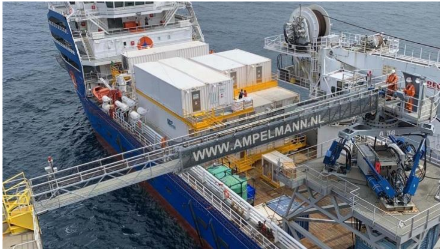
A Service Operation Vessel (SOV) utilising a walk to work system to access another asset (bottom left).
